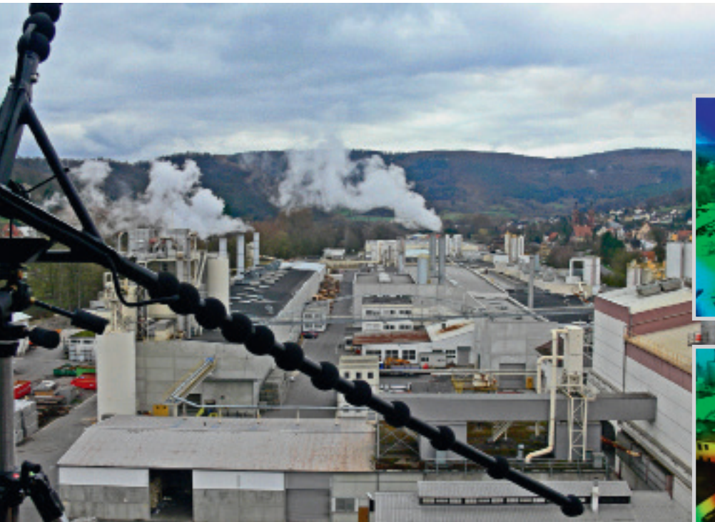
• • • Set-up for acoustic measurement of industrial plant and Acoustic Photos 2D.
